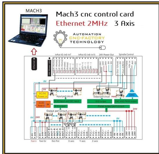
Breakout board cnc Mach3 ETHERNET CNC 24V 3 assi
